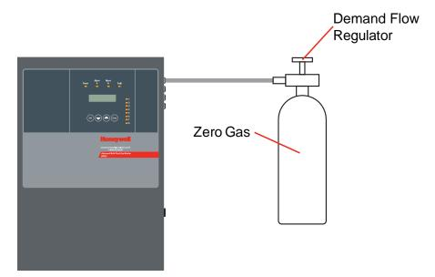
Regardless of gassing configuration, the SQN8x must be in "Calib Zero" mode to zero the unit. **NOTE:**
